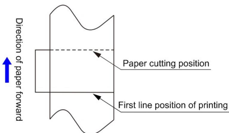
The distance between print head to cutter:  $12.5\text{mm}$
